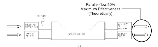
\*\*\*NOTE: This is an example of <u>WHAT NOT TO DO</u>. If the airflows are headed in the same direction, it will work, but not nearly as efficiently.
