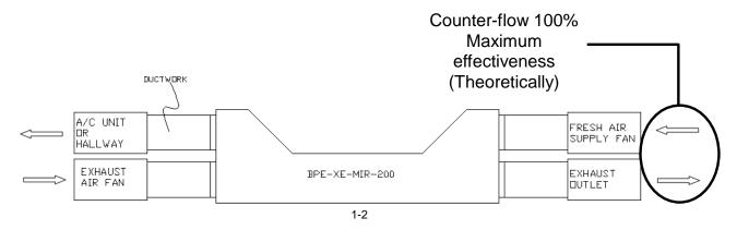
\*\*Note: Exhaust and supply airflows should be counter flow for maximum efficiency.
